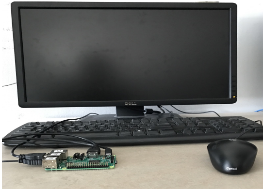
Figure 3. Connecting to a Raspberry Pi using monitor, keyboard, and mouse.
