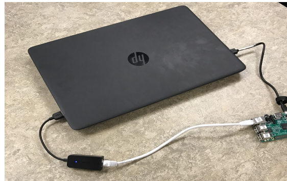
Figure 4. Connecting to a Raspberry Pi using a laptop.
