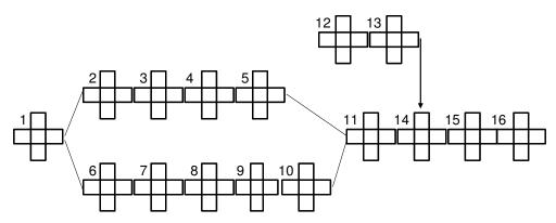
Figure 7: Parallelized Car Restoration Assembly Line with Interior Subassembly
