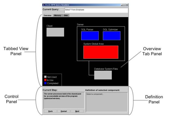
Figure 1: A view of our application's entire GUI, containing the three main panels: *tabbed view panel, control panel,* and *definition panel* along with the *overview tab panel*
