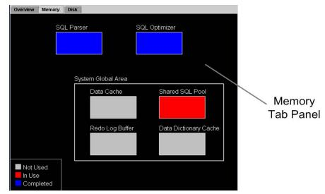
Figure 2: *Memory tab panel* displaying the main memory constructs used in Oracle's DBMS query execution
