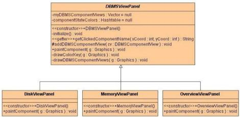
Figure 4: Class diagram for tabbed viewing panels
