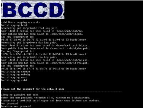
Another part of the initialization process revolves around configuration of the network, which is a critical component to support of distributed computing. Following configuration of the network, the user is prompted to log in with the previously-specified password. Upon logging in for the first time, the user is prompted to start the BCCD *pkbcast* (public key broadcast) program as part of the cluster pre-configuration process.
